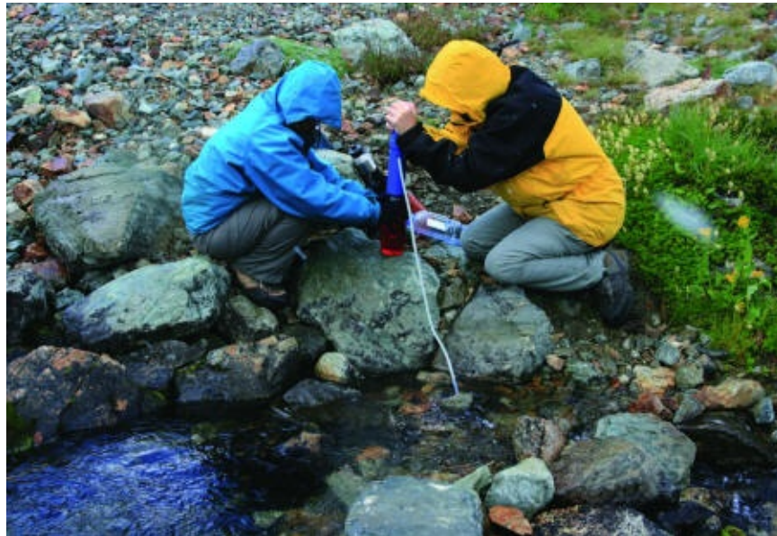
▲ Purifying water with a portable pump filter
