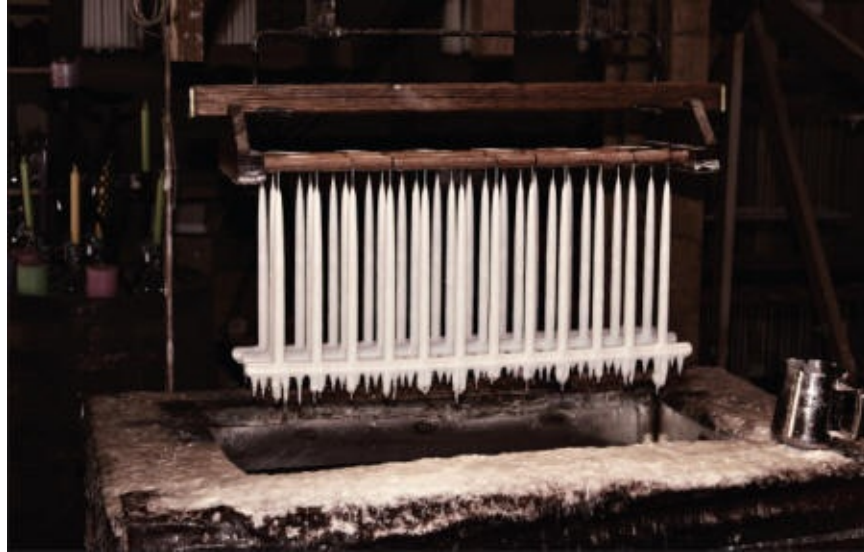
▲ Dipped paraffin candles on a dipping frame
