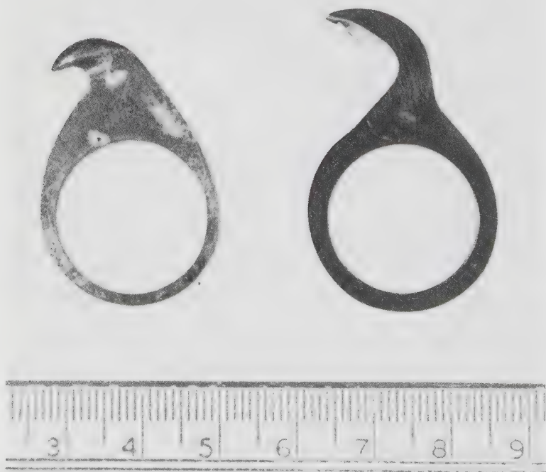
A pair of ring knives with gullet cutter blades. (Photo courtesy of Keith Melton.)
