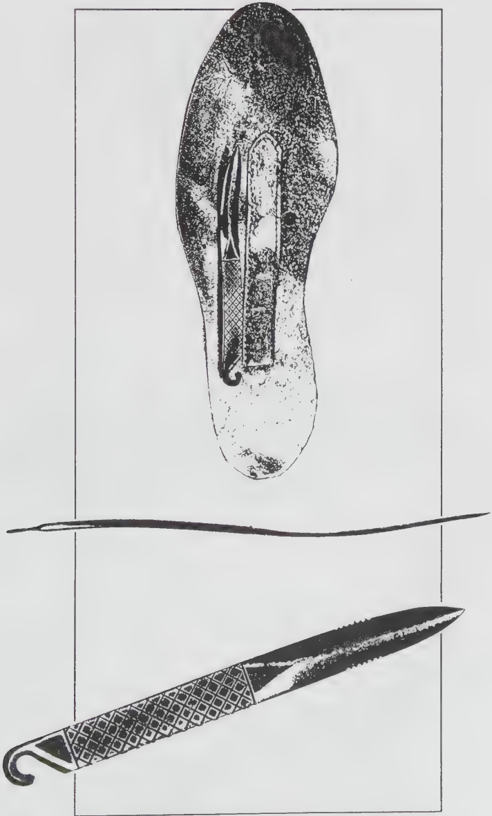
Insole knife with hook cutter. Note how the blade follows the opposite curves of the arch. (Author/Keith Melton illustration.)
